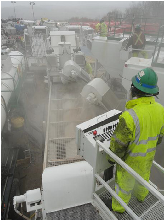
Fig. 4. Worker exposure to silica during hydraulic fracturing. Silica dust created by worker conducting sand transfer operations. Photo shows sand mover and transfer system. (Courtesy of Centers for Disease Control/The National Institute for Occupational Safety and Health (NIOSH).)
